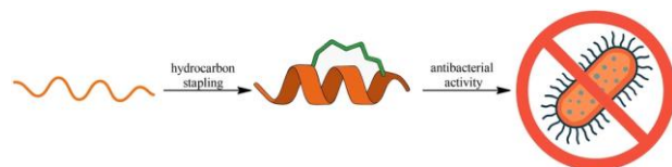
Fig. 1. Schematic representation of the structure–activity relationship for membrane-active peptides. Hydrocarbon stapling stabilizes the \alpha -helical conformation of unstructured, linear peptides thereby conferring antibacterial activity.
