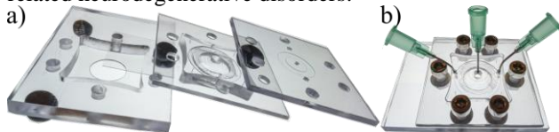
Fig.1. The microfluidic chip. (a) The microfluidic device consists of several layers of polycarbonate that are connected using thin
